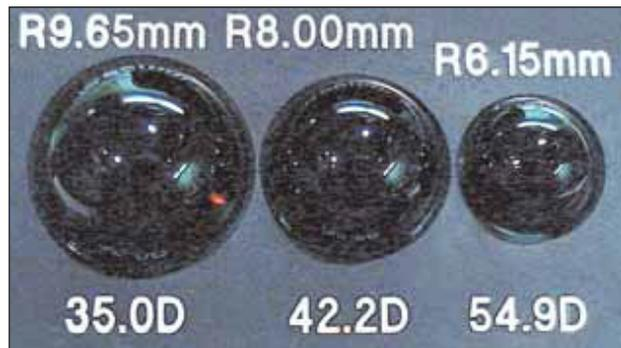
Figure 5. A standard set of calibration spheres (Carl Zeiss Meditec, Inc.). It is important to regularly check the calibration of all instruments used to measure the central corneal power.
